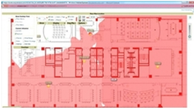
Figure 17 Channel Utilization in VisualRF (Interference)
